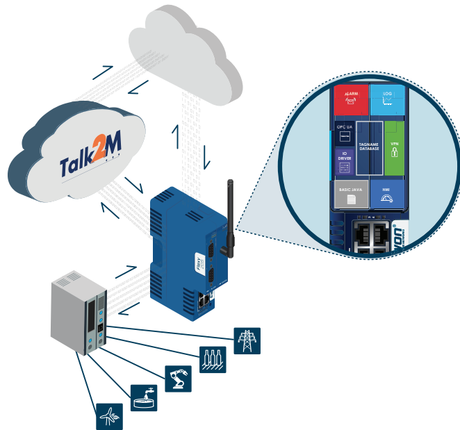
Figure 4-4: The Ewon Flexy connects remote pieces of equipment using different communication protocols.
